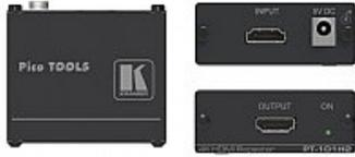
PT-101H2 is a high-performance 4K HDR repeater and extender for HDMI and HDCP 2.2 signals. For 4K@30Hz, it extends the range up to 20m (66ft) (15m to the input, 5m from the output)
